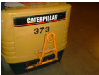
The hitch is attached to the forklift...
